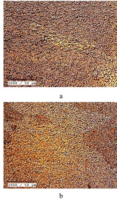
**Fig. 3.** Optical microstructures: a–AA1350 aluminium alloy; b–AA6101-T6 aluminium alloy
