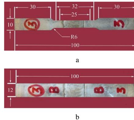
**Fig. 1.** Photographs: a – tensile specimen (ASTM E8M-04 standard); b – bending specimen (ASTM E290-08 standard)
