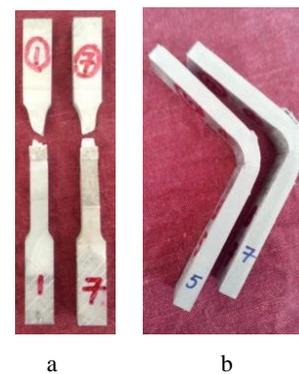
**Fig. 2.** Photographs: a – tensile specimen (after tensile test); b – bending specimen (after bending test)
