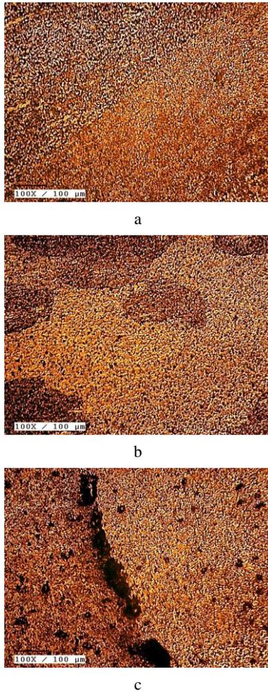
**Fig. 4.** Optical microstructures: a–sample fabricated by 1070 rpm, 78 mm/min and 2°; b–sample fabricated by 765 rpm, 78 mm/min and 0°; c–sample fabricated by 910 rpm, 100 mm/min and 2°
