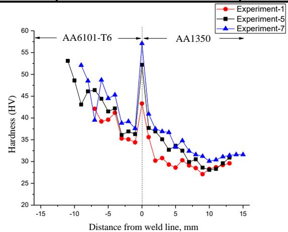
**Fig. 5.** Hardness distribution across the weld
