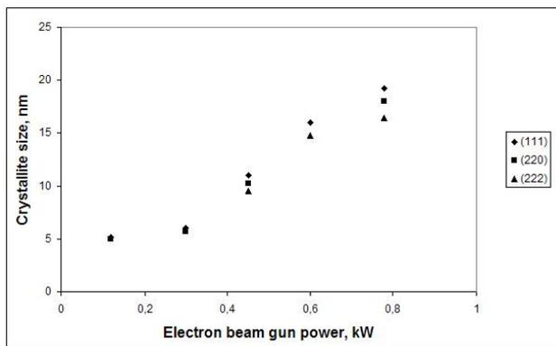
**Fig. 2.** Crystallite size dependence on e-beam gun power of SDC thin films deposited on Alloy 600 (Fe-Ni-Cr) substrate (calculated using Scherrer's equation)
