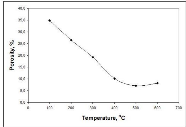
**Fig. 7.** Porosity dependence on substrate temperature of SDC thin films deposited on optical quartz ( $\text{SiO}_2$ ) substrates
