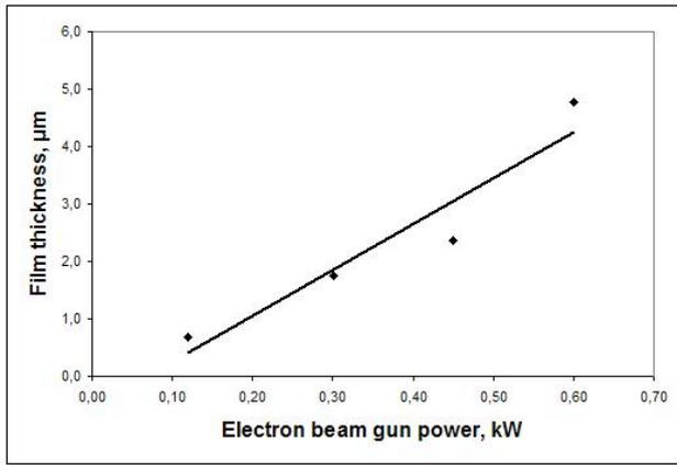
**Fig. 5.** Thickness dependence on e-beam gun power of SDC thin films deposited (deposition time 30 min.) on optical quartz ( $\text{SiO}_2$ ) substrates
