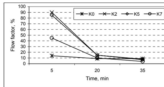
**Fig. 5.** Flow of paste of castables K0, K2, K5 and K7 subject to duration
