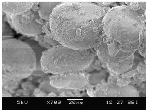
Fig. 1. Structure of the waste FCC catalyst grains
