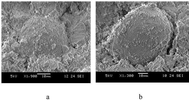
**Fig. 4.** Different structure of matrices of castable with waste catalyst: a – grain of catalyst accrete with binder components, b – lift-off grain
