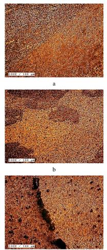
**Fig. 4.** Optical microstructures: a – sample fabricated by 1070 rpm, 78 mm/min and 2°; b – sample fabricated by 765 rpm, 78 mm/min and 0°; c – sample fabricated by 910 rpm, 100 mm/min and 2°
