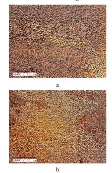
**Fig. 3.** Optical microstructures: a – AA1350 aluminium alloy; b – AA6101-T6 aluminium alloy
