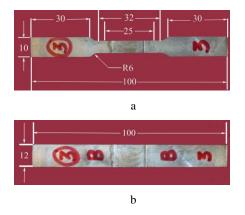
**Fig. 1.** Photographs: a-tensile specimen (ASTM E8M-04 standard); b-bending specimen (ASTM E290-08 standard)
