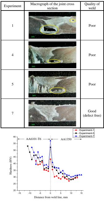
Fig. 5. Hardness distribution across the weld
