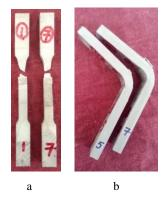
**Fig. 2.** Photographs: a-tensile specimen (after tensile test); b-bending specimen (after bending test)
