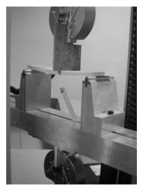
Fig. 1. 3-point bending test
