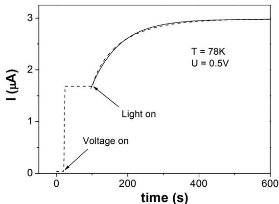
**Fig. 3.** Sample reaction on applied voltage pulse and white light pulse (dashed curve) as indicated on the Figure. The photocurrent growth could be approximated well by exponential dependence as indicated by the solid curve
