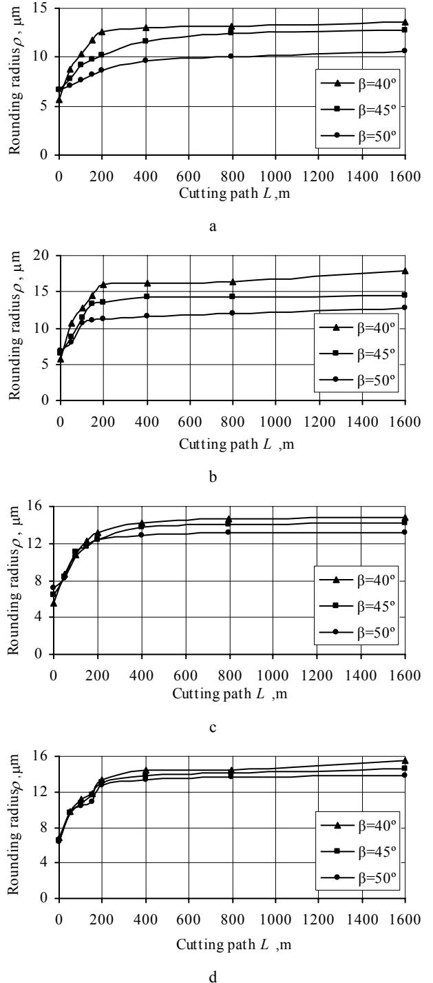
**Fig. 4.** Influence of the cutting path  $L$  on the rounding radius of the cutting edge  $\rho$ : a –  $u_z = 0.5 \text{ mm}$ ; b –  $u_z = 1.0 \text{ mm}$ ; c –  $u_z = 1.5 \text{ mm}$ ; d –  $u_z = 2.0 \text{ mm}$
