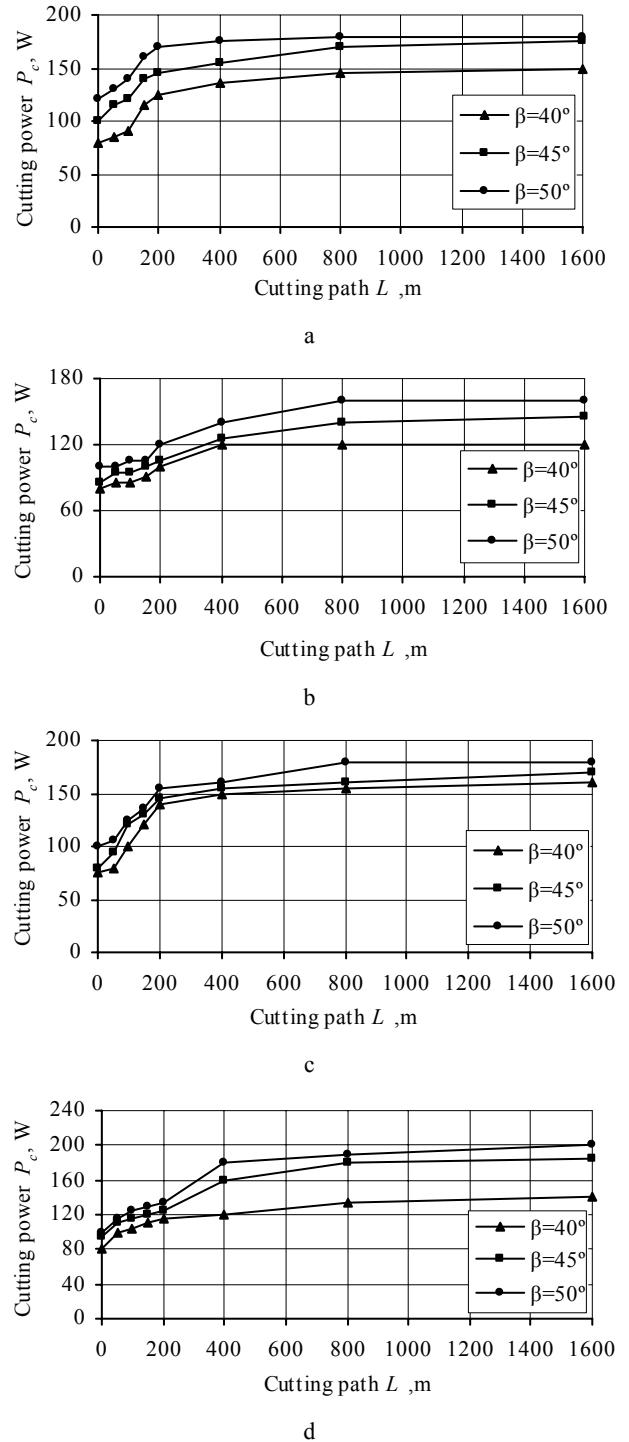
Fig. 5. Influence of the cutting path  $L$  on the cutting power  $P_c$ :
