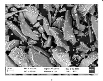
Fig. 1. Microstructure of raw materials: a - clay; b - sand; c - milled glass
