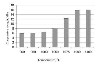
Fig. 3. The influence of burning temperature on compressive strength
