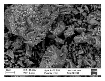
Fig. 4. Microstructure of milled frost resistant porous ceramics samples
