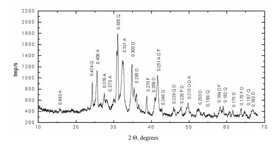
Fig. 5. X-ray diffraction pattern of the sample (as burning temperature is 1100 °C)
