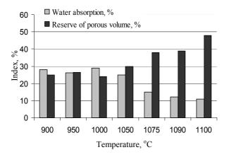
Fig. 2. The influence of burning temperature on water absorption and reserve of porous volume
