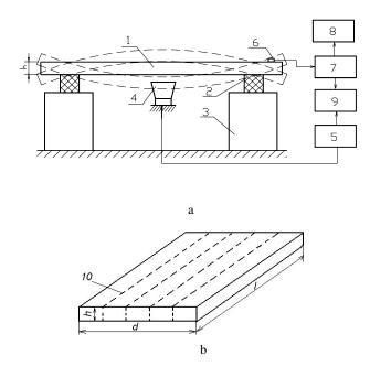
Fig. 2. Schemes of a test stand for wood articles (a) and of board (b): 1 – wood assortment and type of its inflection (mode);
