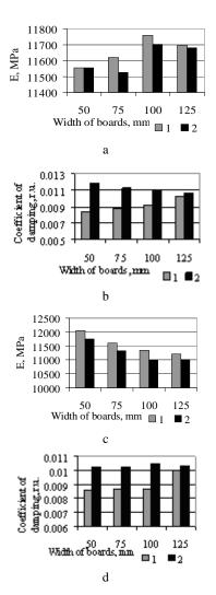
Fig. 4. Variation of modulus of elasticity and coefficient of damping of the boards with tangential cut (a, b) and combined (c, d) cut and their scantlings; where 1 – parameters of uncut board; 2 – average parameters of scantlings forming a respective part of a sample
