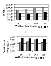
Fig. 3. Variation of modulus of elasticity (a) and coefficient of damping (b) of the boards with radial cut and scantlings forming them: 1 – parameters of uncut boards; 2 – average parameters of scantlings forming some parts of boards
