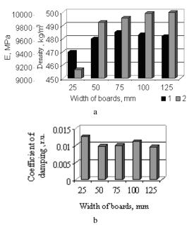
**Fig. 5.** Variation regularities of average density (a, 1), modulus of elasticity (a, 2) and coefficient of damping (b) of the boards with radial cut
