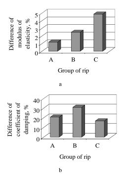
Fig. 6. Values of average differences of modulus of elasticity (a) and coefficient of damping (b) of the boards with radial and combined cuts and their scantlings
