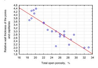
Fig. 2. Ceramic bodies dependence of relative wall thickness of the pores and capillaries on the total open porosity
