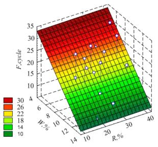
Fig. 6. Tendency of relationship between reserve of pore volume, water absorption and frost resistance determined by oneside method of freezing-thawing
