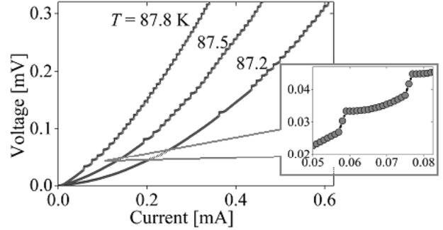
**Fig. 3.** Voltage vs. bias current dependences at  $T = 87.2, 87.5,$  and  $87.8 \text{ K}$  of the LW-bridge at the zero external magnetic field. The inset shows the quasi-Josephson step attributed to entrance of additional vortex – antivortex pair into the channel area at temperature  $T = 87.8 \text{ K}$
