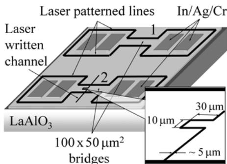
**Fig. 1.** 100- $\mu\text{m}$ -long, 50- $\mu\text{m}$ -wide, and 0.3- $\mu\text{m}$ -thick YBCO bridges laser patterned from a single YBCO film which was deposited onto  $\text{LaAlO}_3$  substrate: 1 – the pristine bridge and 2 – the bridge with LW channel for easy vortex motion
