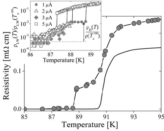
**Fig. 2.** The resistivity versus temperature dependence of a LW-bridge containing a 5- $\mu\text{m}$ -wide channel for easy vortex motion (symbols) and same dependence for pristine sample at 1  $\mu\text{A}$  dc bias. The inset: semilog plots of the normalized resistivity for the LW-bridge at 1, 2, 3, and 5  $\mu\text{A}$  bias currents
