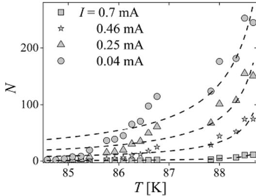
**Fig. 4.** Number  $N$  of vortex-antivortex pairs versus temperature estimated from the  $I$ - $V$  dependences of the LW-bridge at various bias currents and zero external magnetic field. Dashed lines represent best fit of experimental data to inverse of condensation energy of a flux line vs. temperature
