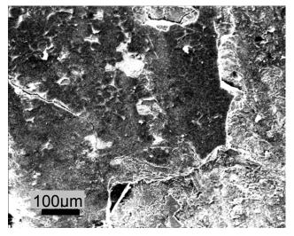
**Fig. 4.** Microstructure of surface of armature rod No 1 affected by lightning discharge picked up by electron scanning microscope SEM EVO 50. Cracks and metal formations are black, non-metal formations – white
