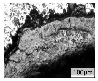
Fig. 3. Microstructure of surface of armature rod No 1 affected by lightning discharge picked up by optical microscope LMA. Etched by 3 % HNO<sub>3</sub> solution in ethanol. Structure: ferrite, pearlite, grey and black formations
