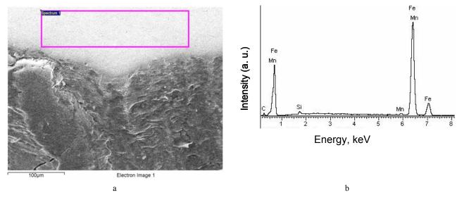
Fig. 5. Influence of lightning discharge on chemical composition of at the surface armature steel rod No 1: a – zone of spectrum analysis; b – spectrum analysis of elemental composition of the main metal. SEM EVO 50 (chemical composition is presented in Table 1)
