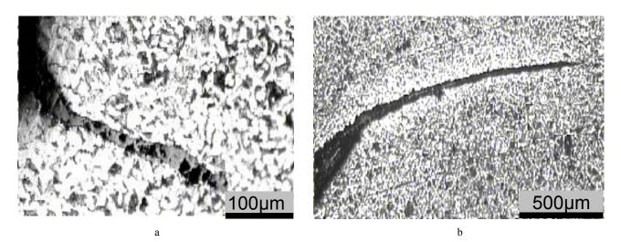
**Fig. 2.** Cracks caused by lightning discharge in armature rods No 1: a – across the rod (magnification ×16); b – along the rod. Etching by 3 % HNO<sub>3</sub> solution in ethanol
