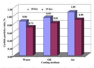
Fig. 3. Carbide particles ratio depended from cooling medium and time of holding
