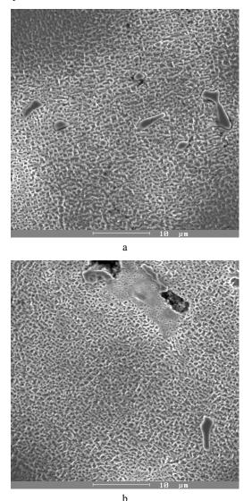
Fig. 5. Superalloy IN 738:  $a - 800^{\circ}$ C/10 hrs. cooled in water,  $b - 800^{\circ}$ C/15 hrs. cooled in water, etch. MARBLE
