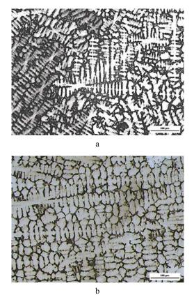
Fig. 4. Superalloy IN 738, secondary dendrite arm spacing: a – starting stage, b – 800 °C/10 hrs. cooled in water, etch. MARBLE
