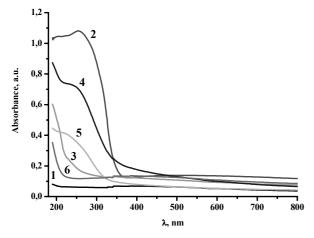
Fig. 1. Optical absorption spectra of the films after heat treatment at 500 °C: 1 – SiO<sub>2</sub>, 2 – TiO<sub>2</sub>, 3 – ZrO<sub>2</sub>, 4 – TiO<sub>2</sub>/ZrO<sub>2</sub>, 5 – SiO<sub>2</sub>/TiO<sub>2</sub>, 6 – SiO<sub>2</sub>/ZrO<sub>2</sub>
