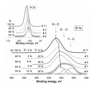
Fig. 6. Detailed XPS O 1s region spectra for sol-gel prepared pure and mixed  $SiO_2$  films (Si 2p region spectra is shown in the inset on the left). At the bottom of picture O 1s spectra of sample # 6 is fitted into three peaks corresponding to the appropriate oxygen bonds as indicated by gray arrows at the top
