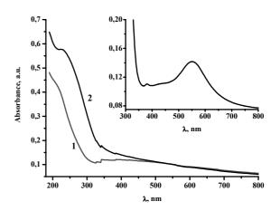
**Fig. 2.** Optical absorption spectra of the films after heat treatment at 500 °C: 1 – TiO<sub>2</sub>/ZrO<sub>2</sub>/SiO<sub>2</sub> (70 % SiO<sub>2</sub>), 2 – TiO<sub>2</sub>/ZrO<sub>2</sub>/SiO<sub>2</sub> (30 % SiO<sub>2</sub>). Inset: TiO<sub>2</sub>/ZrO<sub>2</sub>/SiO<sub>2</sub> (70 % SiO<sub>2</sub>)/ 3.4 % Au film optical absorption spectrum
