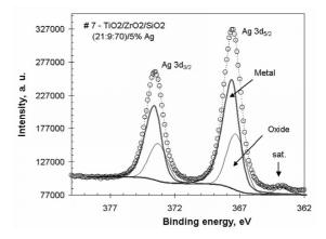
Fig. 10. Fitting procedure for Ag 3d spectra for sample # 7 of mixed oxides film modified with silver nanoparticles TiO<sub>2</sub>/ZrO<sub>2</sub>/SiO<sub>2</sub> (21:9:70)/5 % Ag: circles – experimental data, dashed line – fitted curve; thick line – metallic silver, thin line – silver oxide
