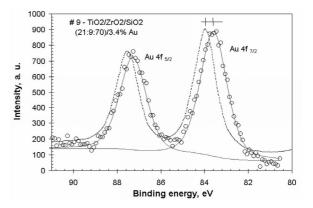
Fig. 11. Fitted Au 4f spectra of sample #9 TiO<sub>2</sub>/ZrO<sub>2</sub>/SiO<sub>2</sub> (21:9:70)/3.4 % Au and gold reference spectra: circles – experimental data, thin lines – fitted curve; dashed line – literature data [17]
