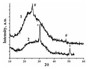
Fig. 3. XRD spectra of  $TiO_2$  (1) and  $ZrO_2$  (2) films deposited onto glass substrates and heat-treated at 600 °C: # –  $TiO_2$ anatase phase related peaks, \* – tetragonal  $ZrO_2$  related peaks
