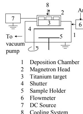
**Fig. 1.** Schematic representation of MS arrangement
