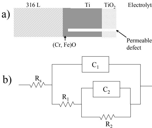
**Fig. 6.** a – Schematic representation of the Ti deposit, b – EEC used in the generation of the simulated data
