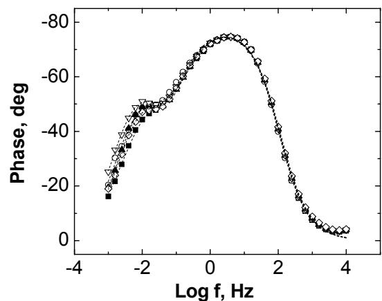
**Fig. 7.** Nyquist and Bode plots of the experimental data for SS and simulated spectra according to the model of Fig. 6, a
