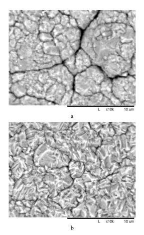
Fig. 2. TTM image of surfaces of Cu (a) and Cu-WC composite (b) coatings
