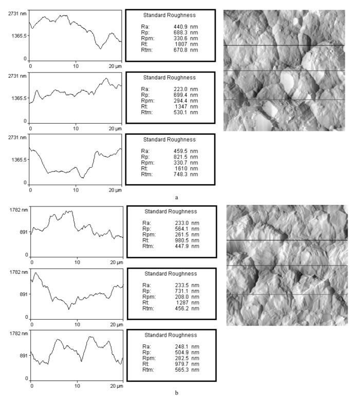
Fig. 5. Analysis data of standard roughness of copper (a) and Cu-WC (b) coatings of various line profile measured by AFM
