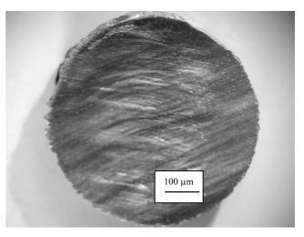
Fig. 4. SMM images of top view of worn surface of Cu-WC coating with a visible twist network of wear tracks at tenfold magnified of real surface
