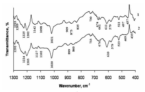
Fig. 1. IR absorption spectra of a PA films treated with 0.004 mol·dm<sup>-3</sup> solution of H<sub>2</sub>S<sub>12</sub>O<sub>6</sub> at 10 °C different time. Sulfurization time, h: 1 - 2, 2 - 6
