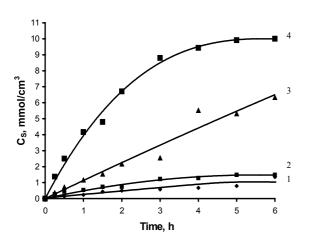
Fig. 5. Change of sulfur concentration in PA with time during its treatment with 0.004 mol·dm<sup>-3</sup> solution of  $H_2S_{12}O_6$  at different temperatures. The temperature (°C) of  $H_2S_{12}O_6$  solution: 1 - 10, 2 - 20, 3 - 30, 4 - 40
