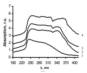
**Fig. 4.** UV absorption spectra of PA films treated 1.5 h with 0.004 mol·dm<sup>-3</sup> solution of  $H_2S_{12}O_6$  at different temperature. Sulfurization temperature, °C: 1 – 10, 2 – 20, 3 - 30, 4 - 40
