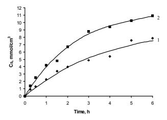
Fig. 6. Change of sulfur concentration in PA with time during its treatment with the solution of  $H_2S_{12}O_6$  of different concentration at the temperature of 40 °C. Concentration, mol·dm<sup>-3</sup>: 1 - 0.002, 2 - 0.004
