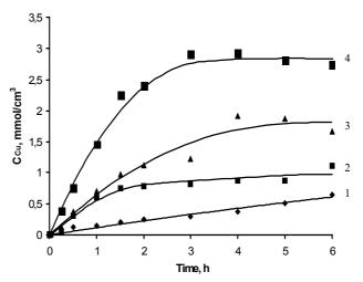
Fig. 7. Dependence of the concentration of copper in sulfide layer on PA film on sulfurization time when treating it with  $0.004 \text{ mol} \cdot \text{dm}^{-3}$  solution of  $\text{H}_2\text{S}_{12}\text{O}_6$  at different temperatures. The temperature (°C) of  $\text{H}_2\text{S}_{12}\text{O}_6$  solution: 1 - 10, 2 - 20, 3 - 30, 4 - 40
