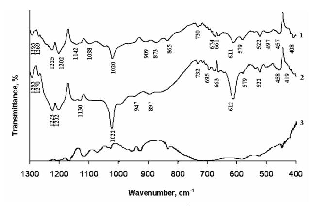
Fig. 2. IR absorption spectra of a PA films treated during 2 h with 0.004 mol·dm<sup>-3</sup> solution of  $H_2S_{12}O_6(1, 2)$  and of initial untreated PA (3). PA treatment with  $H_2S_{12}O_6$  temperature, °C: 1 – 10, 2 – 20
