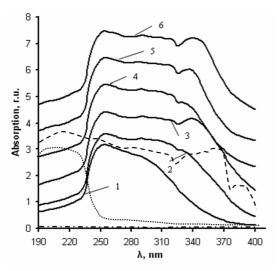
**Fig. 3.** UV absorption spectra of PA films (..... – without compensation,  $-\cdot - \cdot -$  using PA absorption compensation), PA films treated with 0.004 mol·dm<sup>-3</sup> solution of H<sub>2</sub>S<sub>12</sub>O<sub>6</sub> at 20 °C different time and of the 0.004 mol·dm<sup>-3</sup> solution of H<sub>2</sub>S<sub>12</sub>O<sub>6</sub> – ---. Sulfurization time, h: 1 – 0.25, 2 – 0.5, 3 – 1.5, 4 – 3.0, 5 – 4.0, 6 – 5.0
