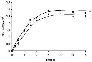
Fig. 8. Dependence of the concentration of copper in sulfide layer on PA film on sulfurization time when treating it with solution of  $H_2S_{12}O_6$  of different concentration at the temperature of 40 °C. Concentration, mol·dm<sup>-3</sup>: 1 – 0.002, 2 – 0.004
