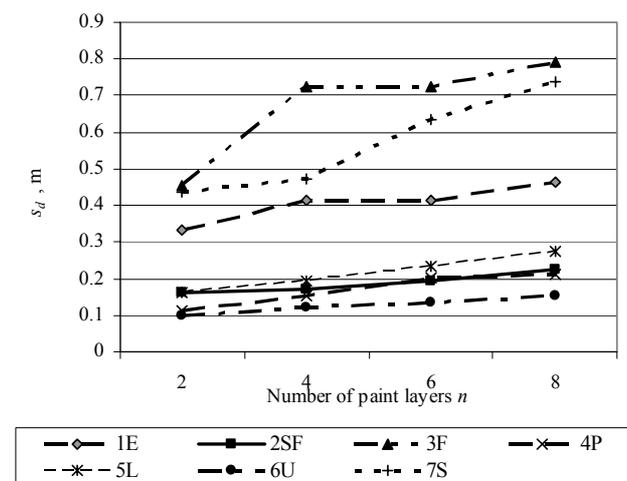
**Fig. 1.** Dependence of the thickness of the air layer  $s_d$  equivalent to the paint coating's water vapour permeability on the number of the paint layers. Paint marks: 1E – silicate 1; 2SF – siloxan; 3F – acrylic 1; 4P – polyurethane; 5L – siloxan-acrylic; 6U – silicate 2; 7S – acrylic 2
