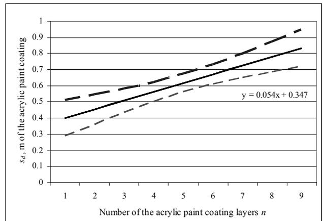
**Fig. 6.** The reliable interval of the dependence of the thickness of the air layer  $s_d$  equivalent to the acrylic paint coating's water vapour permeability on the mean of the number of paint layers
