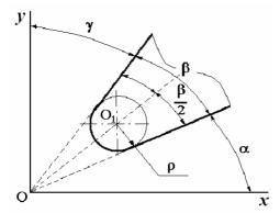
Fig. 2. Microgeometrical parameters of the cutting tool
