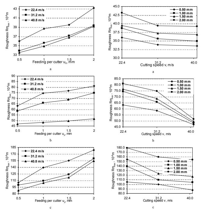
**Fig. 3.** Influence of feed per cutter  $u_z$  (mm) for different cutting speed (22.4; 31.2 and 40.8 m/s) on the roughness of processed surface  $Rm_{max}$  (μm):  $a - \rho = 6.57$  μm;  $b - \rho = 20.4$  μm;  $c - \rho = 40.0$  μm
