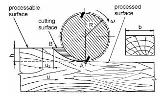
Fig. 1. Technological scheme of longitudinal milling [1]
