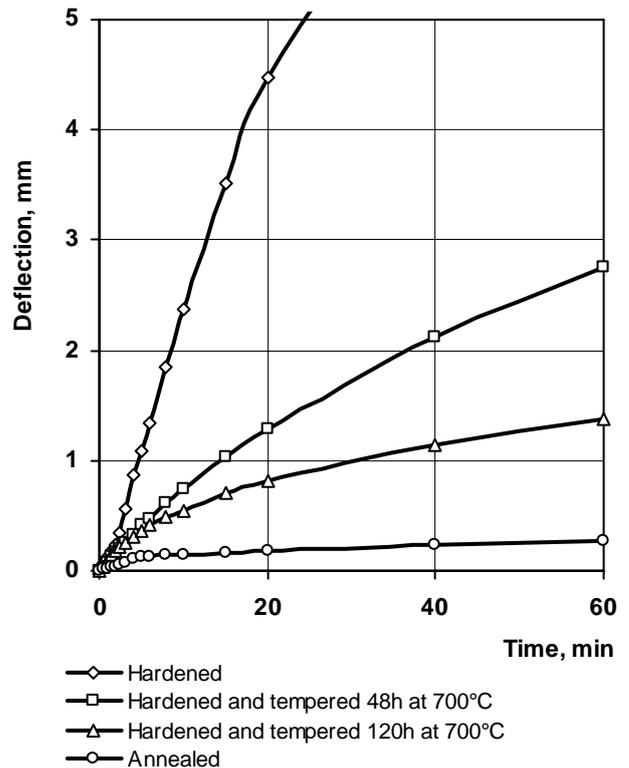
Fig. 5. Dependence of steel 12XH3A plasticity on structural state during tempering at 650 °C temperature. Bending stress 90 N/mm<sup>2</sup>
