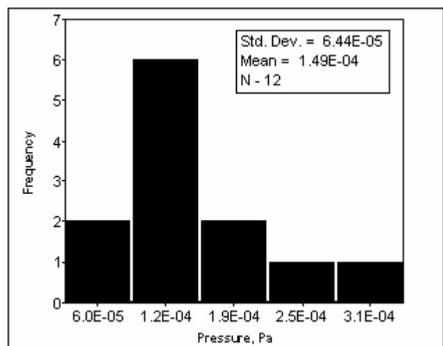
Fig. 7. Histogram of 12 A33EKC CCR tubes total pressures
