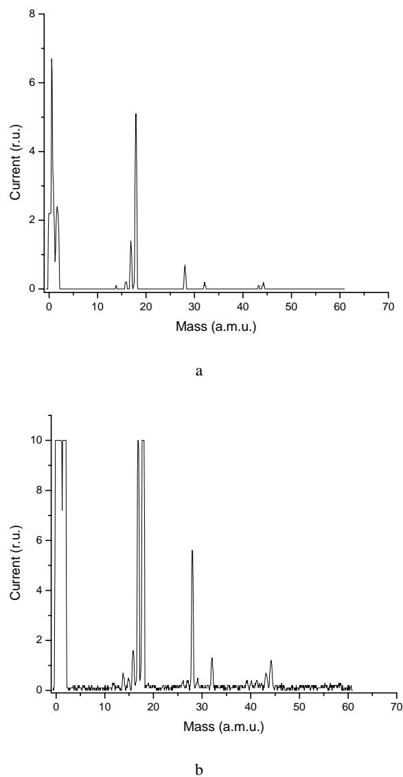
**Fig. 2.** Typical CCRT residual gas mass spectra, measured for A33EKC class tubes. Sensitivity factor of a device is:
