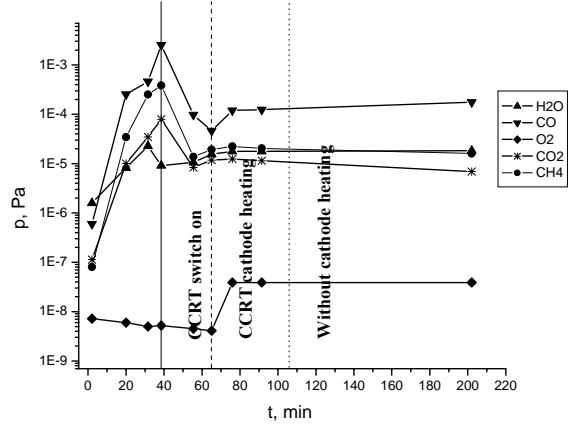
**Fig. 5.** Residual gases (H<sub>2</sub>O, CO, CO<sub>2</sub>, CH<sub>4</sub>) partial pressures dependence on time
