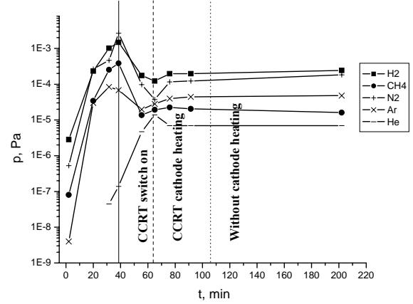
**Fig. 4.** Residual gases (H<sub>2</sub>, CH<sub>4</sub>, N<sub>2</sub>, Ar, He) partial pressures dependence on time
