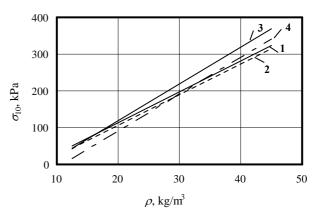
Fig. 4. The empirical lines of the values of stress corresponding to 10 % deformation of expanded polystyrene slabs under compression, depending on their density. Lines 1, 2 – mean and predicted stress values for slabs manufactured by Lithuanian enterprices; 3, 4 – the same according to the data provided in [7]
