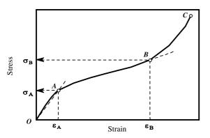
Fig. 1. A scheme of expanded polystyrene under short-term compression [3 – 5]
