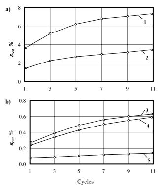
**Fig. 2.** The develomment of residual deformations in expanded polystyrene with the density of  $14 \text{ kg/m}^3$ : a – under cycling compressive stress equal to:  $1 - \sigma_{10}$ ;  $2 - \sigma_5$ , b – the same for:  $3 - 1.2\sigma_{cr}$ ;  $4 - \sigma_{cr}$ ;  $5 - 0.8\sigma_{cr}$
