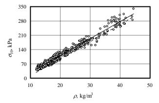
Fig. 3. The stress corresponding to 10% deformation of expanded polystyrene slabs under compression, depending on their density. o – experimental values; the continuous line – the empirical regression line of the mean stress value according to slab density; the dotted line – the same for the predicted stress value according to the slab density
