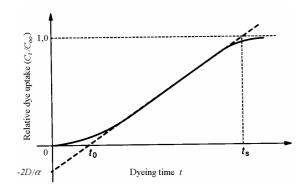
**Fig. 1.** The surface barrier effect in wool dyeing [1]
