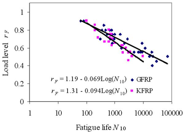
Fig. 12. Wöhler curves of the GFRP and KFRP laminates
