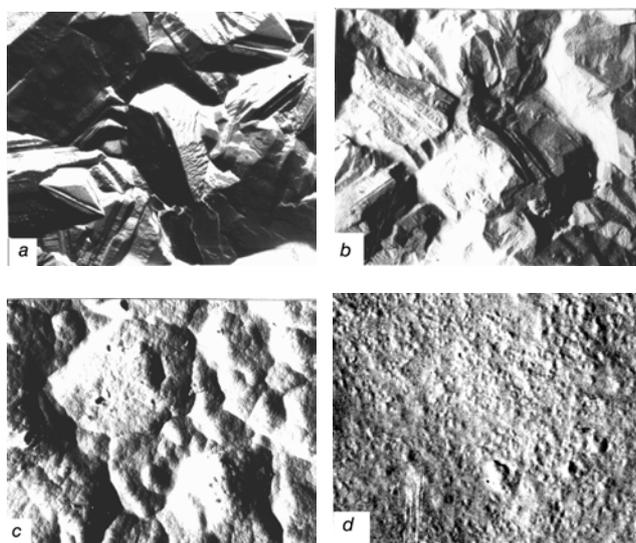
**Fig. 4.** Micrographs of silver electrodeposits on velour Cu underlayer obtained by SEM: a – velour Cu underlayer, b – a + 1  $\mu\text{m}$  Ag, c – a + 5  $\mu\text{m}$  Ag, d – a + 20  $\mu\text{m}$  Ag;  $i_k = 1 \text{ A/dm}^2$ . Magnification: a, b, c –  $\times 6000$ , d –  $\times 12000$
