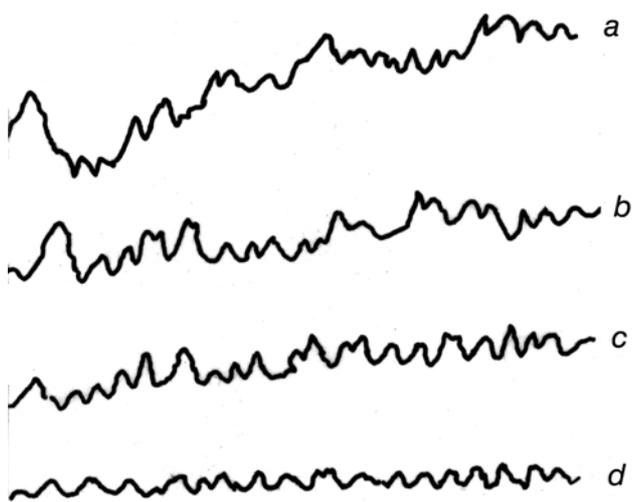
**Fig. 3.** Profilograms of silver deposits on velour copper: a – velour Cu underlayer of the thickness of 15  $\mu\text{m}$ , b – a + 0.5  $\mu\text{m}$  Ag, c – a + 1  $\mu\text{m}$  Ag, d – a + 5  $\mu\text{m}$  Ag;  $i_k = 1 \text{ A/dm}^2$ . 1.5 mm in vertical direction correspond to 0.2  $\mu\text{m}$  while in horizontal – 5  $\mu\text{m}$
