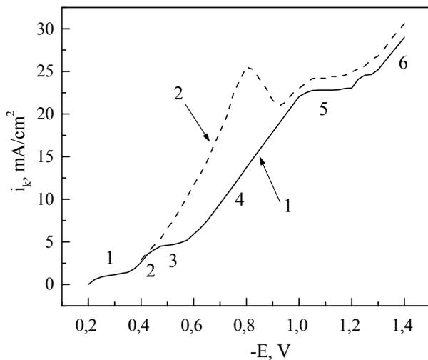
**Fig. 1.** The dependence of silver cathode potential  $E$  on the cathode current density  $i_k$  in various electrolytes (g/l): 1 –  $\text{KAg}(\text{CN})_2$  – 55,  $\text{KSCN}$  – 250,  $\text{K}_2\text{CO}_3$  – 20; 2 – (the same as for 1) +  $\text{KNaC}_4\text{H}_4\text{O}_6 \cdot 4\text{H}_2\text{O}$  – 50,  $\text{Sb}\{\text{K}(\text{SbO})\text{C}_4\text{H}_4\text{O}_6 \cdot 1/2\text{H}_2\text{O}\}$  – 1.5,  $\text{Na}$  ricinolate – 1
