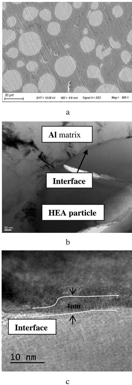
**Fig. 3.** Micrographs for the hot-pressed composites with 30 vol.% of HEA reinforcement: a–SEM micrographs; b–the interface between the HEA particle and the Al metal matrix; c–the interface at a higher magnification
