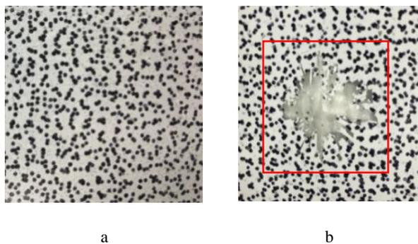
**Fig. 10.** The effect of composite plates after the second impact: a – with SMA wires; b – without SMA wires
