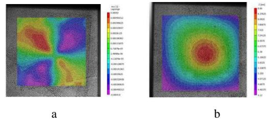
Fig. 5. Impact response cloud of composite plates (example): a—xy plane strain cloud; b—deflection cloud
