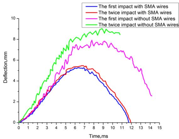
Fig. 7. Deflection of composite plates impacted by two times
