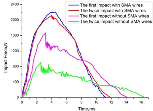
Fig. 6. Impact forces of composite plates impacted by two times
