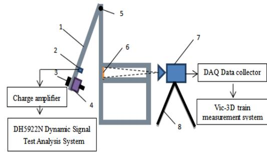
Fig. 2. Composite plate impact test schematic
