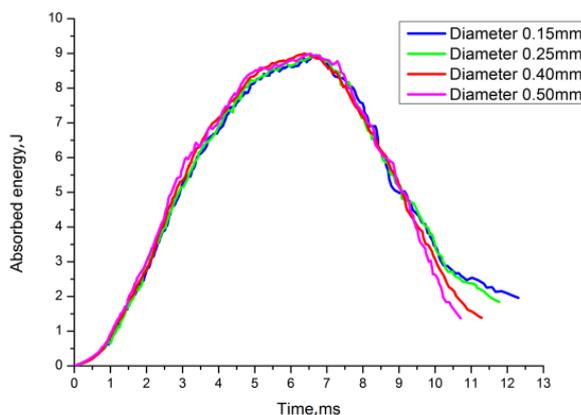
**Fig. 13.** Absorbed energy of composite plates with different diameter SMA wire
