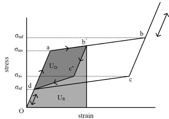
**Fig. 1.** Strain energy absorbed by SMA
