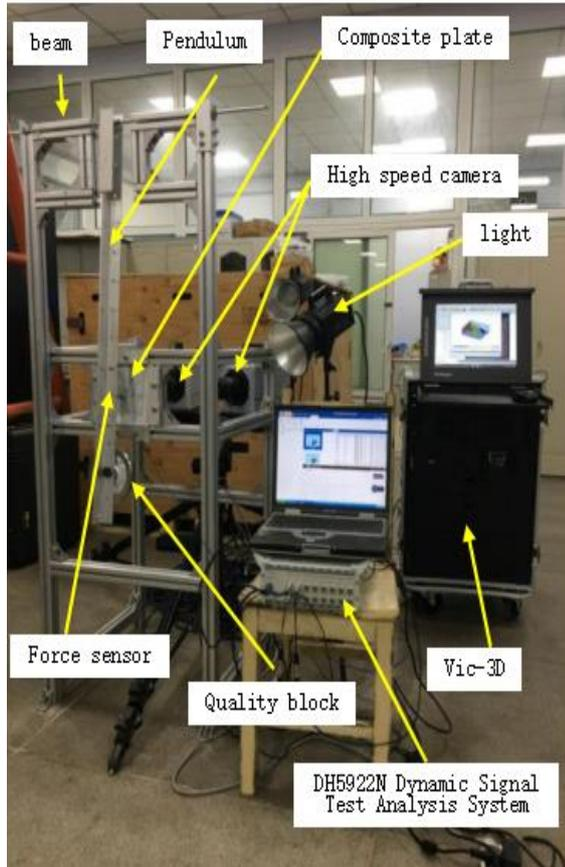
Fig. 3. Composite plate impact test bench
