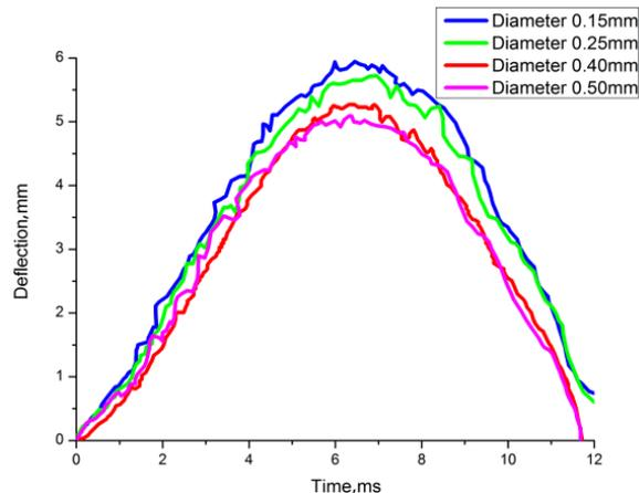
**Fig. 12.** Deflection of composite plates with different diameter SMA wires
