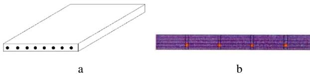
Fig. 4. Composite plate schematic: a—sketch map; b—specific laying position of SMA wire
