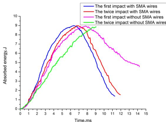
Fig. 8. Absorbed energy of composite plates impacted by two times
