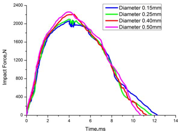
**Fig. 11.** Impact forces of composite plates with different diameter SMA wires
