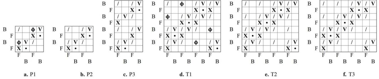
Fig. 1. Weave plans of designed self-stitched double fabrics
