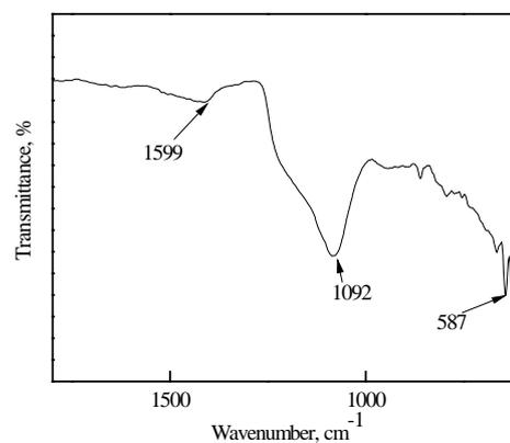
**Fig. 2.** FT-IR spectrum of  $\text{Fe}_3\text{O}_4@\text{SiO}_2$  materials
