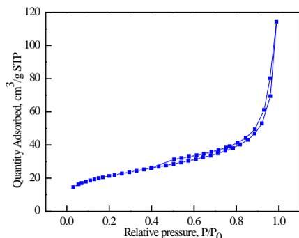
**Fig. 8.** The N<sub>2</sub> adsorption-desorption isotherm of F@S@m-S-4.78 materials
