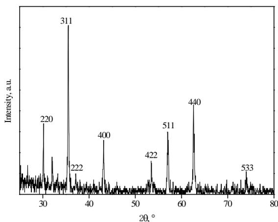
**Fig. 1.** The X-ray diffraction pattern (XRD) of particles
