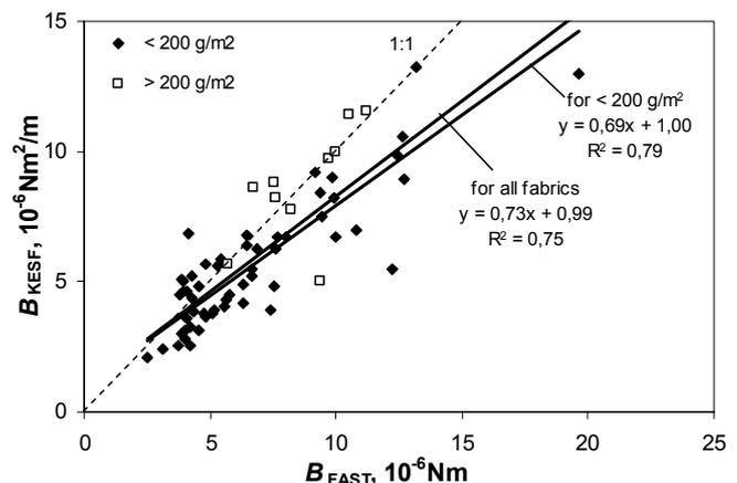
Fig. 11. The relationships between KES-F and FAST bending rigidity values for all analysed fabrics and light-weight (< 200 g/m<sup>2</sup>) fabrics
