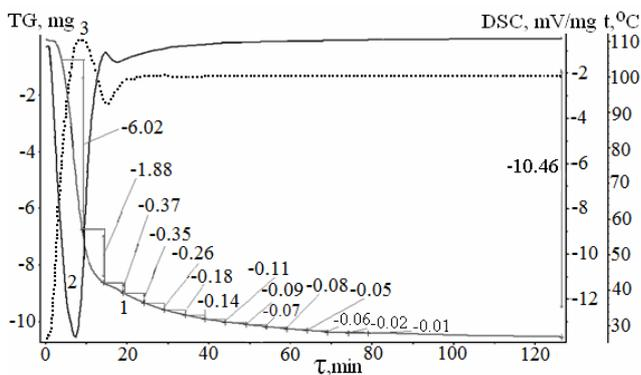
**Fig. 10.** Regeneration of Al<sub>2</sub>O<sub>3</sub>-Cact at 100 °C: 1 – TG curve, 2 – DSC curve, 3 – temperature rise curve
