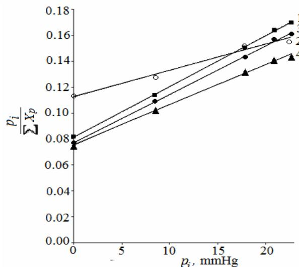
**Fig. 9.** Linear dependence for calculation of  $X_m$  and adsorption coefficient  $b$ : 1 – Al<sub>2</sub>O<sub>3</sub>-(B-2), 2 – Al<sub>2</sub>O<sub>3</sub>-(WS-42), 3 – Al<sub>2</sub>O<sub>3</sub>-(WS-42A), 4 – Al<sub>2</sub>O<sub>3</sub>-(OU)
