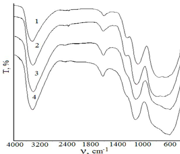
**Fig. 6.** IR patterns for various  $\text{Al}_2\text{O}_3\text{-C}_{\text{act}}$  derivatives: 1 –  $\text{Al}_2\text{O}_3\text{-(WS-42A)}$ , 2 –  $\text{Al}_2\text{O}_3\text{-(B-2)}$ , 3 –  $\text{Al}_2\text{O}_3\text{-(OU)}$ , 4 –  $\text{Al}_2\text{O}_3\text{-(WS-42)}$
