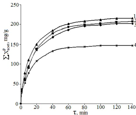
**Fig. 7.** Kinetic curves of acetone vapor adsorption at 22 °C, 748 mmHg–763 mmHg, air humidity 40 %–45 % for various adsorbents: 1 –  $\text{Al}_2\text{O}_3\text{-(OU)}$ , 2 –  $\text{Al}_2\text{O}_3\text{-(B-2)}$ , 3 –  $\text{Al}_2\text{O}_3\text{-(WS-42A)}$ , 4 –  $\text{Al}_2\text{O}_3\text{-(WS-42)}$
