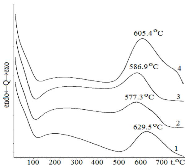
Fig. 3. DSC curves of  $\text{Al}_2\text{O}_3\text{-C}_{\text{act}}$  at air atmosphere: 1 –  $\text{Al}_2\text{O}_3\text{-(WS-42A)}$ , 2 –  $\text{Al}_2\text{O}_3\text{-(B-2)}$ , 3 –  $\text{Al}_2\text{O}_3\text{-(WS-42)}$ , 4 –  $\text{Al}_2\text{O}_3\text{-(OU)}$
