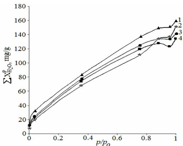
**Fig. 8.** Water vapor adsorption isotherms at 25 °C: 1 – Al<sub>2</sub>O<sub>3</sub>-(OU), 2 – Al<sub>2</sub>O<sub>3</sub>-(WS-42A), 3 – Al<sub>2</sub>O<sub>3</sub>-(B-2), 4 – Al<sub>2</sub>O<sub>3</sub>-(WS-42)
