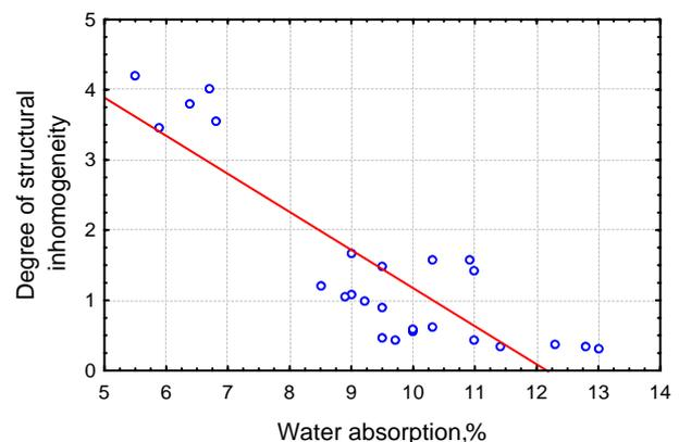
**Fig. 3.** Ceramic bodies dependence of water absorption on the degree of structural inhomogeneity
