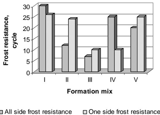
Fig. 4. Frost resistance of ceramic bodies measured by all-side and one-side method of freezing-thawing
