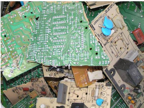
**Fig. 1.** Preliminarily crushed PCBs separated from dismantled post-consumer electronic equipment
