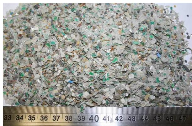
Fig. 5. Separated non-ferrous metals and composite plastic from the coarse fraction +1.25–2.5 mm
