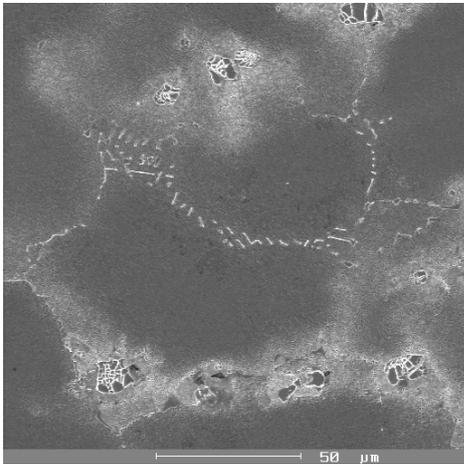
Fig. 1. Superalloy IN 738: starting stage, etch. Marble, SEM
