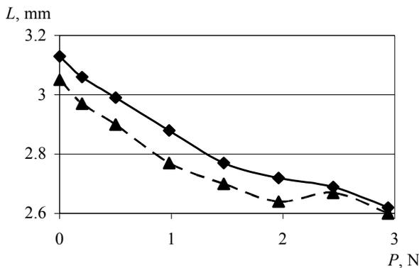
Fig. 4. Dependence of the stitch length  $L$  upon two-sided load  $P$  and pressing force, when rotational frequency of the main shaft is  $1100 \text{ min}^{-1}$  and external friction force of fabric is  $13.7$  (— —  $45 \text{ N}$ , - - - -  $85 \text{ N}$ )
