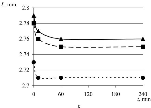
**Fig. 2.** Dependence of plain weave fabric the stitch length  $L(x)$  upon internal friction ( $tg\delta$ ) and time  $t$ , when rotational frequency of the main shaft is the following: a –  $200 \text{ min}^{-1}$ , b –  $1100 \text{ min}^{-1}$ , c)  $2100 \text{ min}^{-1}$  (---- 0.03, — — 0.033, ---- 0.037)
