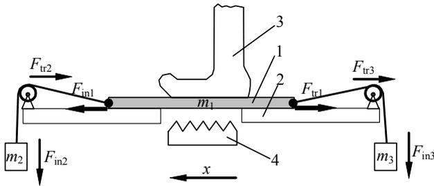
**Fig. 1.** Diagram of sewing garment feeding and acting forces: 1 – sewing garment, 2 – needle plate, 3 – presser foot, 4 – toothed plate;  $m_1, m_2, m_3$  – masses of elements of the sewing garment and loads;  $F_{in1}$  – inertial force of the sewing garment;  $F_{in2}, F_{in3}$  – inertial forces of load elements,  $F_{tr1}$  – friction force between the sewing garment and a needle plate and presser foot,  $F_{tr2}, F_{tr3}$  – friction forces acting in fair – leads,  $x$  – axis
