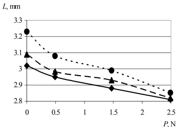
Fig. 5. Dependence of the stitch length  $L$  upon two-sided load  $P$  and rotational frequency of the main shaft, when pressing force is  $45 \text{ N}$  and external friction force of fabric is  $10.9 \text{ N}$  (— —  $200 \text{ min}^{-1}$ , - - - -  $1100 \text{ min}^{-1}$ , ·····  $2100 \text{ min}^{-1}$ )
