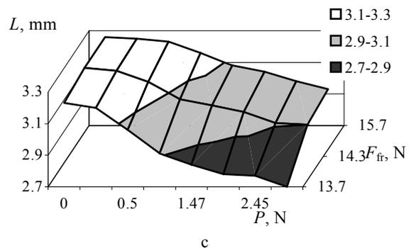
**Fig. 3.** Dependence of the stitch length  $L$  upon external friction force of fabric  $F_{fr}$  and two-sided load  $P$ , when pressing force is 45 N and rotational frequency of the main shaft is the following: a –  $200 \text{ min}^{-1}$ , b –  $1100 \text{ min}^{-1}$ , c –  $2100 \text{ min}^{-1}$
