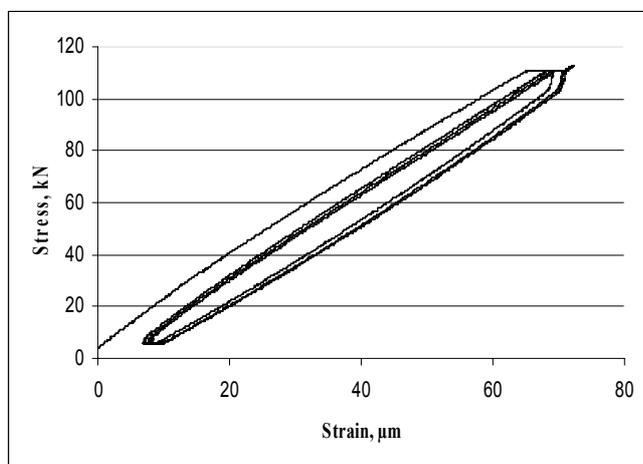
**Fig. 2.** Stress-strain relationship for concrete with rubber waste
