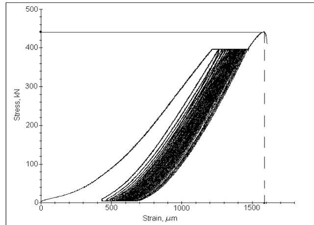
**Fig. 6.** Stress-strain relationship of the concrete with rubber waste additive after 20 cycles loading 90 percent of compressive strength
