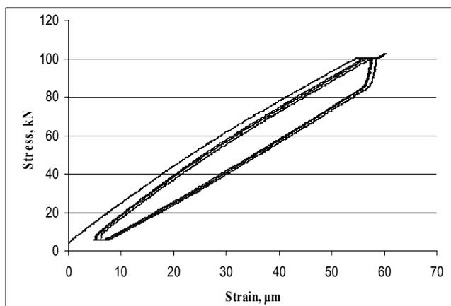
**Fig. 1.** Stress-strain relationship for concrete without rubber waste
