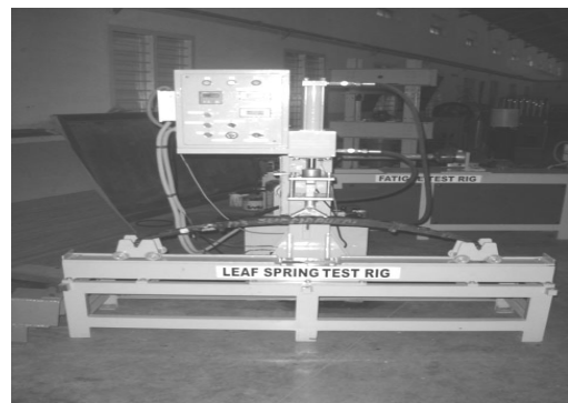
Fig. 4 (c). Static load test for steel leaf spring
