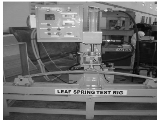
Fig. 4 (a). Static test of composite mono leaf spring
