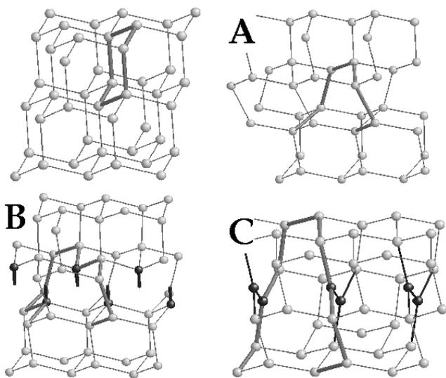
**Fig. 1.** Ball-and-stick representation of the perfect zinc-blende structure (upper left) and of three different relaxed configurations for perfect screw dislocations. The grey thick sticks show the Burgers circuit for each core. Black spheres are atoms with dangling bonds (B) or with hybridization  $sp^2$  (C)
