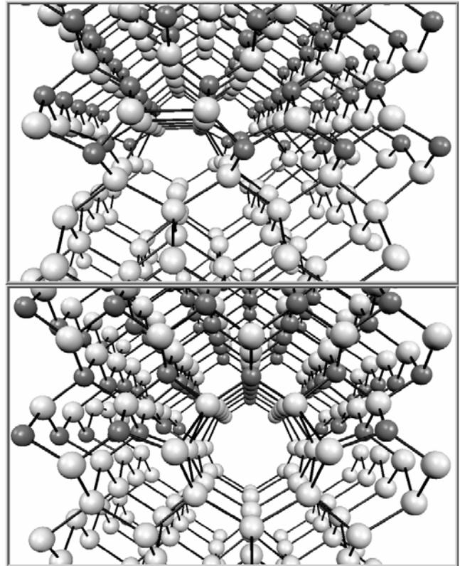
**Fig. 3.** Ball-and-stick representation along directions [110] (up) and [1-10] (down) of the most stable atomic configuration calculated for the SiC/Si(001) interface. Light grey (dark grey) spheres represent silicon (carbon) atoms
