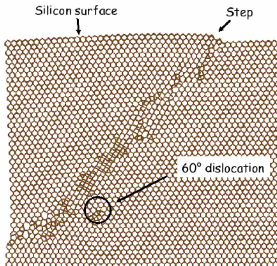
**Fig. 2.** Cross-section view of a silicon surface with a monoatomic step, submitted to a uniaxial compression of 10% (disoriented by  $22.5^\circ$  with respect to the step line), after relaxation at 0K
