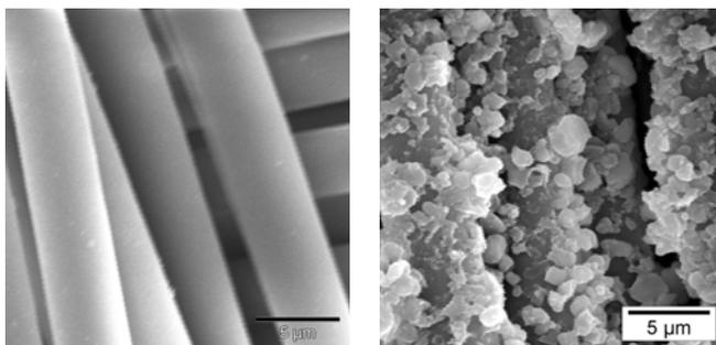
**Fig. 4.** SEM micrographs of proton conducting membranes (taken from edge): Glass composite membrane: blank (left micrograph) and after impregnation with ZP (right micrograph)
