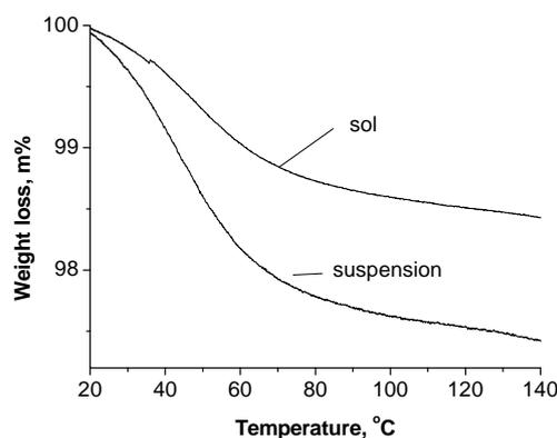
**Fig. 3.** Thermogravimetric analysis of the membrane impregnated with zirconium phosphate from ZrO<sub>2</sub> sol and suspension
