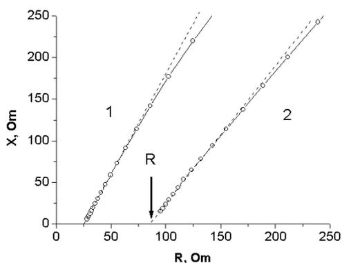
**Fig. 2.** Cole-Cole plots for membrane after 3<sup>rd</sup> (2) and 4<sup>th</sup> (1) impregnation with zirconium phosphate from ZrO<sub>2</sub> sol (where R- volume resistance)
