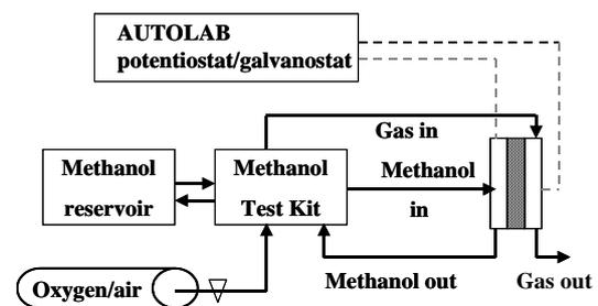
Fig. 1. Experimental set-up for DMFC testing
