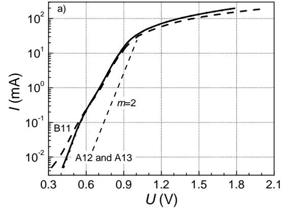
**Fig. 5.** Current-voltage characteristics for DFB lasers: sample A12 without ageing and burned-in lasers A13 and B11
