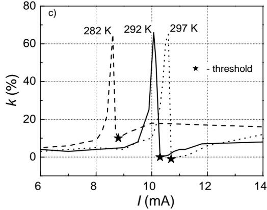
**Fig. 4.** Correlation factor between optical and electrical noise signals in the frequency range 10 Hz – 20 kHz dependencies on laser current in the threshold region at different temperatures (sample A12)
