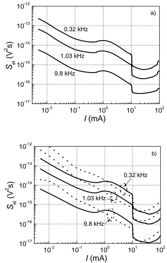
**Fig. 6.** Electrical fluctuation spectral density dependencies on laser current for investigated DFB lasers at three frequencies (0.32 kHz, 1.03 kHz and 9.8 kHz): a) sample A12 without ageing; b) burned-in samples A13 (solid line), and B11 (dot line)
