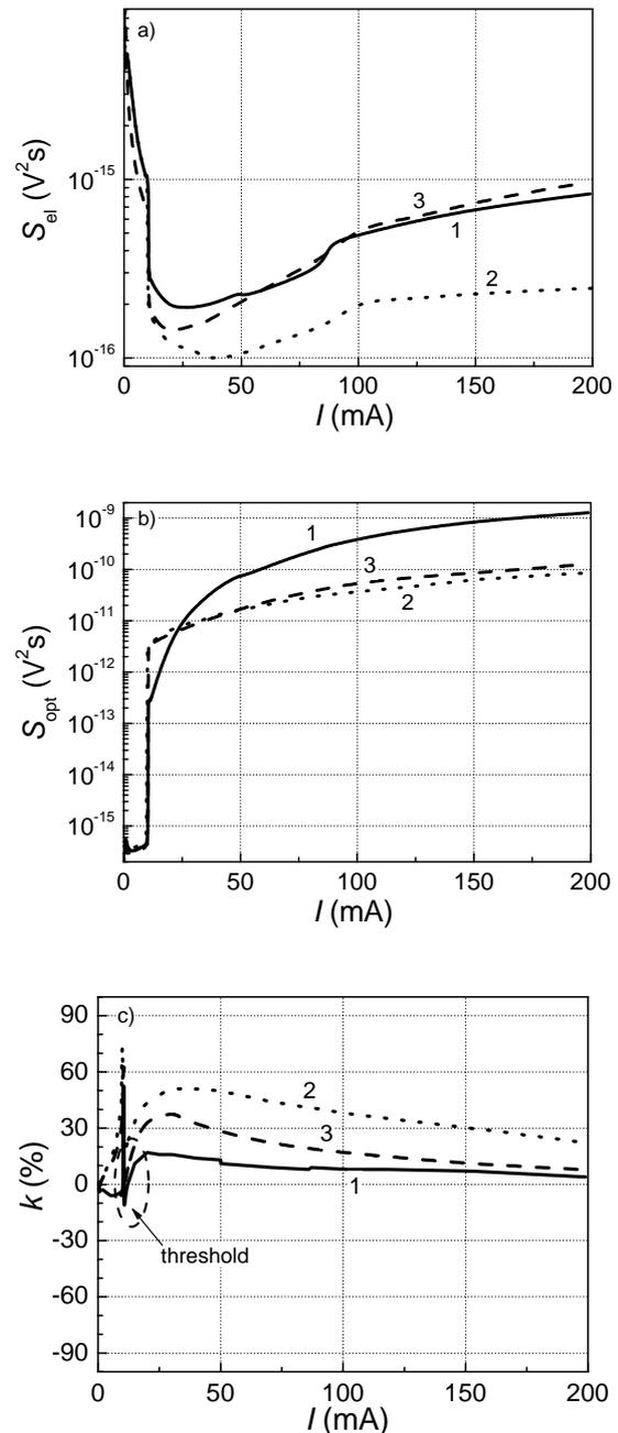
**Fig. 3.** Low-frequency noise characteristics for the investigated DFB lasers: a – electrical and b – optical fluctuation spectral density at 1.03 kHz, and c – correlation factor between optical and electrical noise signals in the frequency range 10 Hz – 20 kHz dependencies on laser current (curve 1 – not aged sample A12 (solid line), curve 2 – burned-in sample A13 (dot line), and curve 3 – burned-in sample B11 (dashed line))
