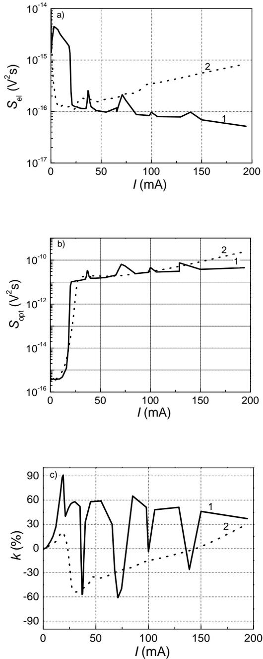
**Fig. 1.** Low-frequency noise characteristics of the FP lasers: a – electrical and b – optical fluctuation spectral density at 1.03 kHz, and c – correlation factor between optical and electrical noise signals in the frequency range 10 Hz – 20 kHz dependencies on laser current: sample A03 without facet coating (curve 1 – solid line), and sample B02 with facet coating (curve 2 – dot line)
