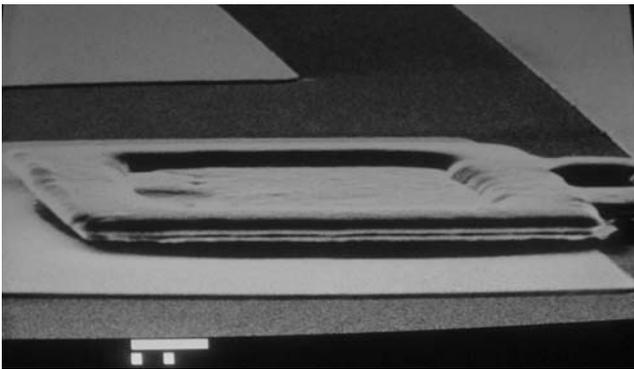
**Fig. 4.** Cantilever beam support area. Mark size 10  $\mu\text{m}$
