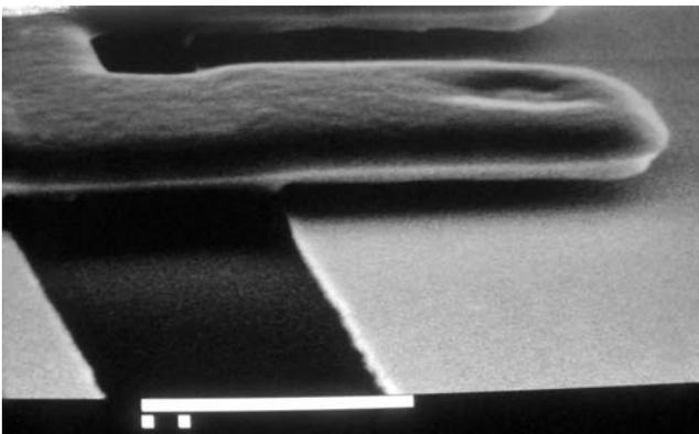
**Fig. 5.** Contact tip gap. Mark size 10  $\mu\text{m}$
