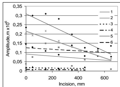
Fig. 5. Changes in panel vibration shift amplitudes: 1 – panel I, 64 – 93 Hz frequency range; 2 – panel I, 264-268 Hz; 3 – panel II, 83 – 184 Hz; 4 – panel II, 521 – 524 Hz; 5 – panel III, 45 – 77 Hz; 6 – panel III, 274 – 277 Hz
