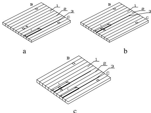
Fig. 2. Scheme of glued solid wood panels and modeled defects: a – defect modeled at the edge of the panel; b – in the centre of the panel; c – at the edge and in the centre of the panel; 1 – solid wood scantling, 2 – glue line, 3 – defect; l – incision length, A, B, C – characteristic panel zones
