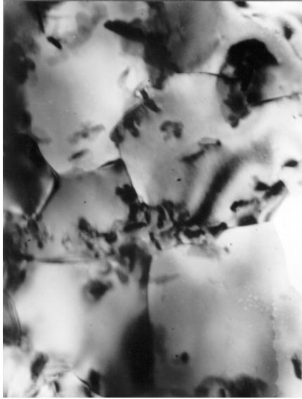
Fig. 6. Submicrostructure (foil) material Al-12Al 4 C 3 - transverse direction
