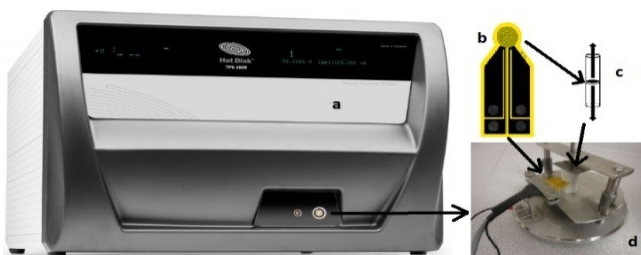
Fig. 4. a–the real time picture of device; b–Kapton sensor; c–one dimensional mode specimen geometry; d–measurement set up
