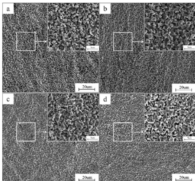
**Fig. 6.** Surface morphology characteristics of new martensitic heat-resistant steel after high temperature oxidation in air at 700 °C for different time: a–30 h; b–80 h; c–140 h; d–200 h
