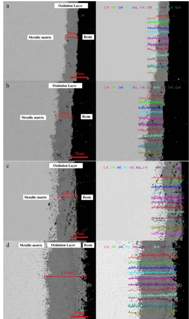
**Fig. 8.** Cross-section morphology and EDS analysis of new martensitic heat-resistant-steel after high temperature oxidation in air at 700 °C for different time: a-30 h; b-80 h; c-140 h; d-200 h
