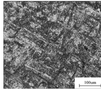
**Fig. 2.** Microstructure of new martensitic heat resistant steel
