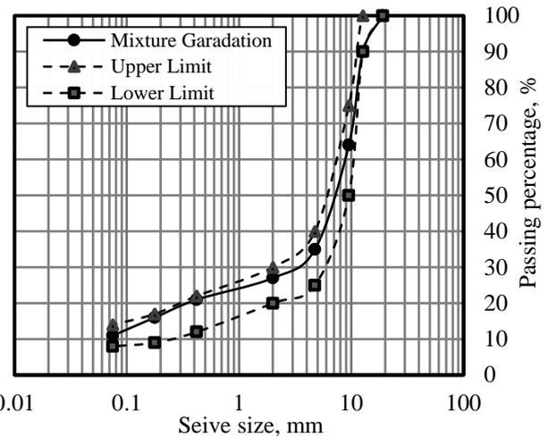
**Fig. 1.** Aggregate gradation and specification limits for SMA mixture
