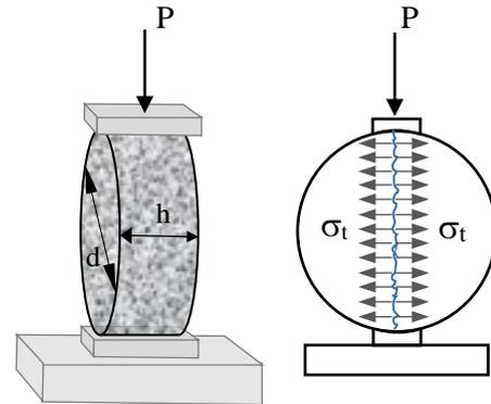
**Fig. 2.** Indirect tensile strength test loading condition
