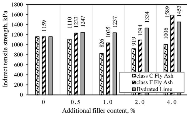
Fig. 4. Indirect tensile test results for dry method
