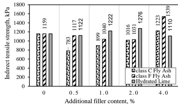
Fig. 5. Indirect tensile test results for wet method
