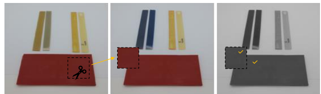
Fig. 3. The reference sample (left) and sample under treatment (middle), treated sample with a grayscale mask and adjusted luminosity (right). The selected area for the adjustment of luminosity is shown in all images
