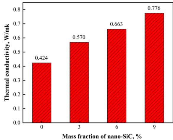
**Fig. 8.** Thermal conductivity of different composite PCMs
