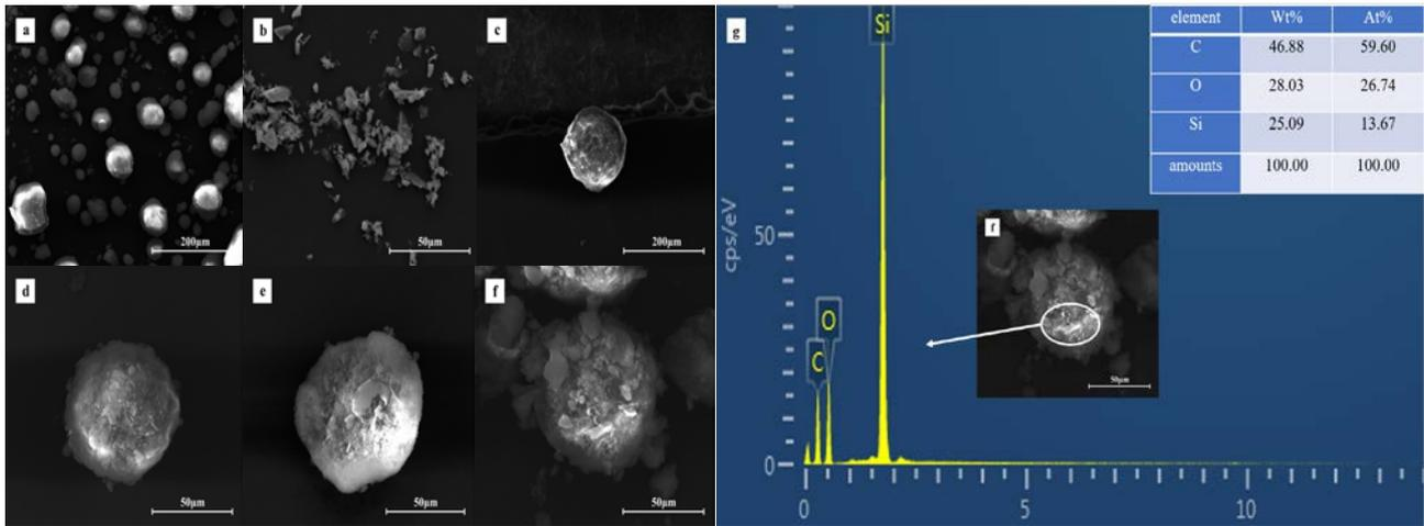
**Fig. 3.** ESEM photographs of different composite PCMs: a – nano-SiO<sub>2</sub>; b – nano-SiC; c – SPCM3; d – CPCM1; e – CPCM2; f – CPCM3 and EDS spectra of CPCM3
