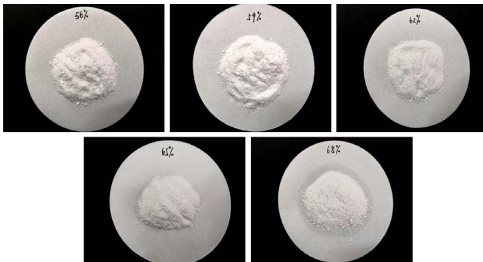
**Fig. 2.** Leakage tests of the MA-PA/nano-SiO<sub>2</sub> composites with different MA-PA content
