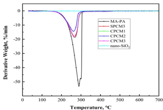
**Fig. 7.** DTG curves of MA-PA, nano SiO<sub>2</sub>, SPCM3, CPCM1, CPCM2 and CPCM3
