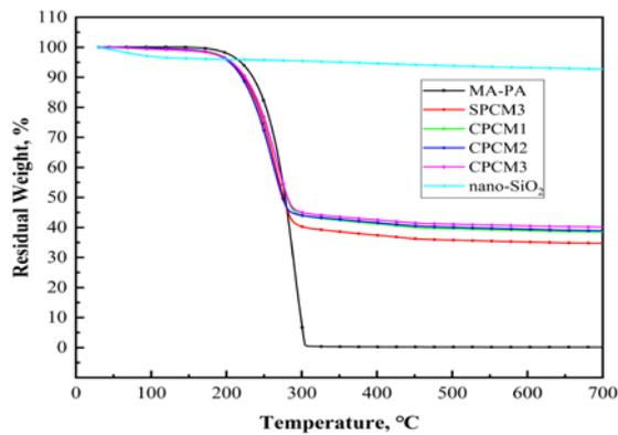
**Fig. 6.** TGA curves of MA-PA, nano-SiO<sub>2</sub>, SPCM3, CPCM1, CPCM2 and CPCM3
