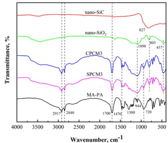
**Fig. 4.** FT-IR spectra of nano-SiC, nano-SiO<sub>2</sub>, MA-PA, SPCM3 and CPCM3
