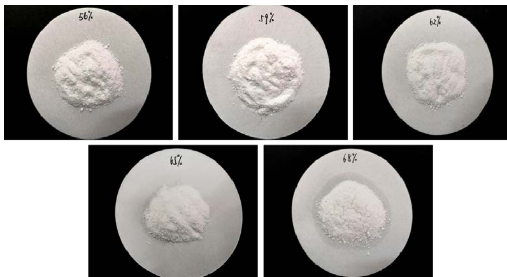
Fig. 2. Leakage tests of the MA-PA/nano-SiO 2 composites with different MA-PA content
