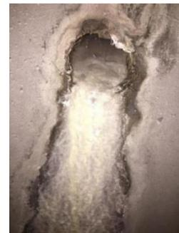
**Fig. 3.** Crystal blockage of a drainage pipe
